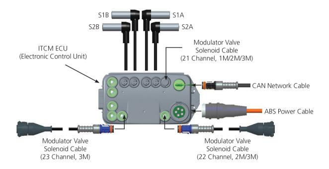
**Note:** If 2S/1M is desired, use Sensors (S1A and S1B). Use blanking plugs in un-used Sensor Connections.
